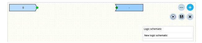
Every input, output or logical block is clearly colour coded on the connectors, indicating which data type can be connected. Green means a binary input (1 or 0), blue a numeric value and yellow a textual value. Outgoing connectors are lighter in colour and an incoming connector is darker in colour. Logical blocks can only be connected to connectors of the same type. You can connect up to 10 lines to one connector (incoming or outgoing).
